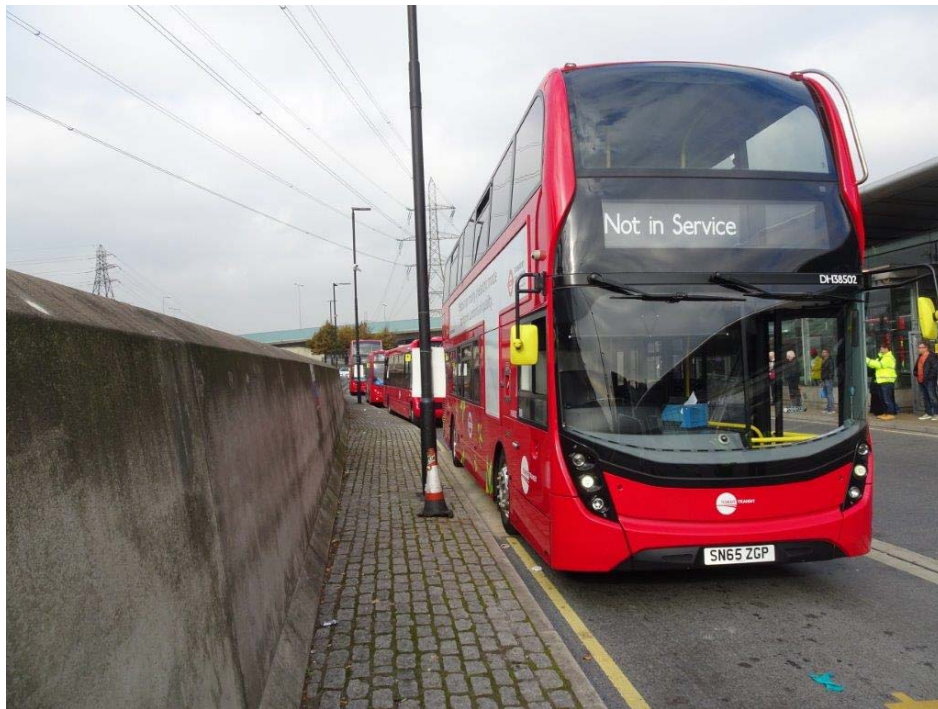
Figure 1: Bus Bay at Canning Town with the bus lowered over the induction pad.
