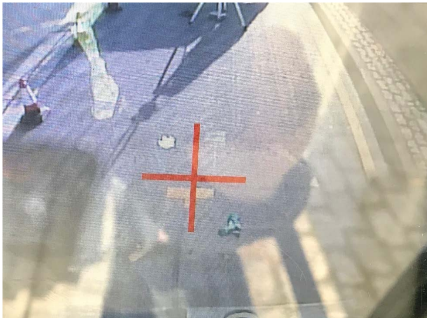
Figure 7: Alignment Camera screen in bus
