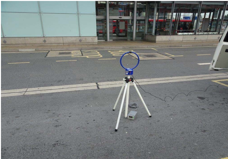
Figure 3: Loop orientation for maximum received signal from the induction pads.
